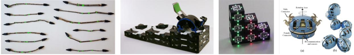
Figure 2.2: Illustrative examples along the range of construction material capability. From left to right: found material (sticks) from Devin Carroll; co-designed building blocks in the TERMES system from [17]; ‘stigmergic’ smart building blocks from [26]; and the ATRON modular robot from [15].
